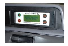
2 Action Switch on Tipper Control Unit, message will display...
