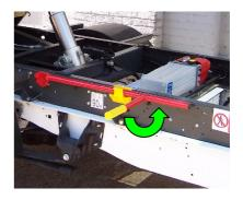
Do not leave the vehicle with the body raised and propped for any length of time. The protective oil film on the ram will evaporate, drain away or be washed away. Corrosive elements may erode the highly finished surface of the ram, which in turn could lead to damage of the ram seals, resulting in potential oil leaks.
