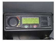
**2** Action Switch on Tipper Control Unit, message will display...
